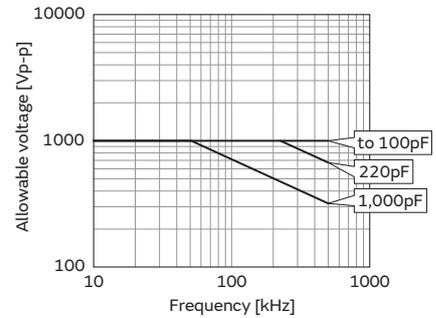
The sine-wave frequency VS allowable voltage
