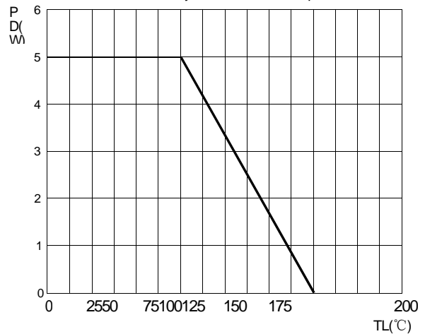
图6: 功率损耗曲线 FIG6: Steady State Power Dissipation
