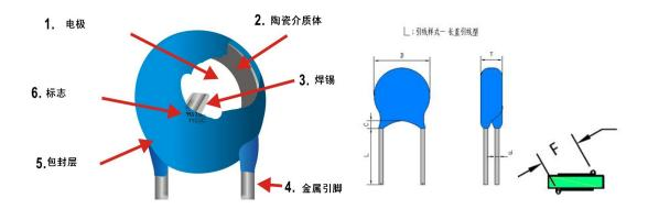
Note: The coating layer is epoxy resin coating, and the color is blue;
